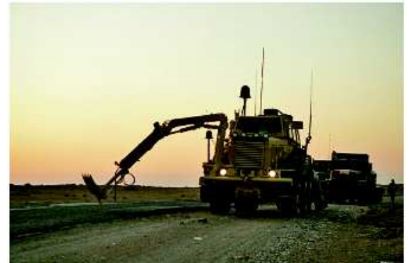
U.S. Marines assigned to 9th Engineer Support Battalion (ESB), 1st Naval Construction Regiment, use the arm of a Buffalo mine-protected vehicle to clear a hole during a route repair mission near Lake Habbaniyah on Nov. 1, 2008. Part of 9th ESB's mission during Operation Iraqi Freedom is to improve road conditions for the Iraqi people and coalition forces.
